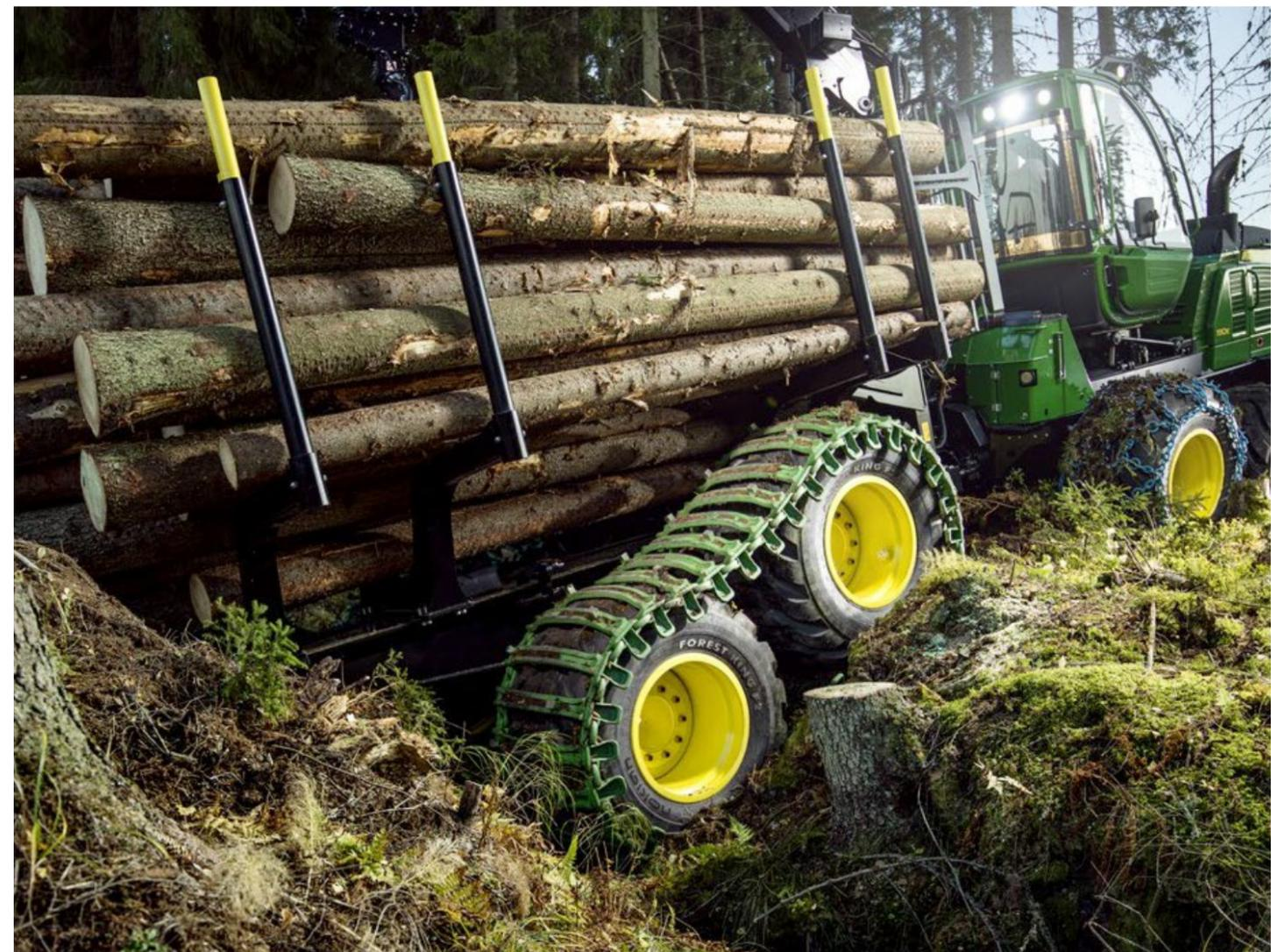
*the right proportion of steel belts providing the tire the capacity to withstand lower pressure with no performance loss – allow forestry tires to “float” better, causing lower soil compaction and withstanding harsh work conditions. “It’s also worth mentioning that forestry tires have tread designs with special slots for use with tracks. This means it’s possible to get the*
