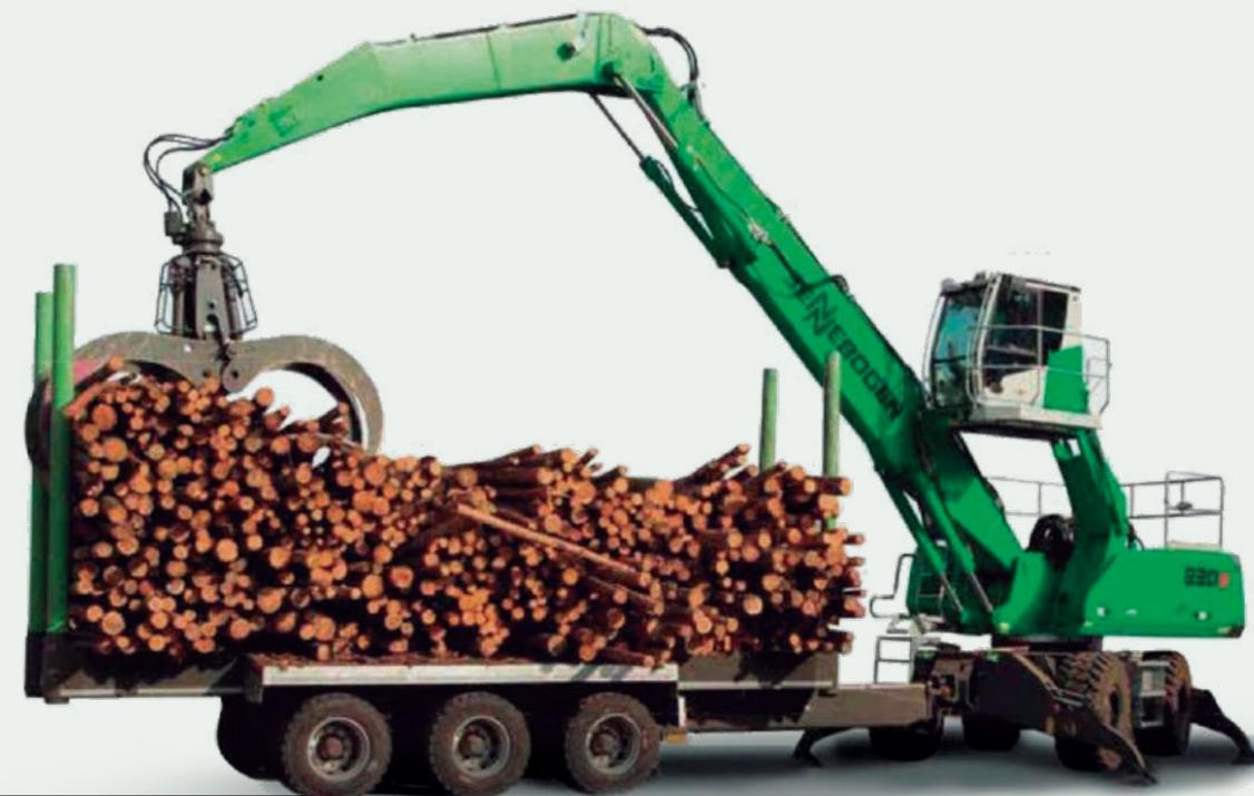
*meters high with logs 7 meters long. The material handlers are suitable machines for this type of operation, allowing the operator to have total control of the operation, with safety and visibility.*
